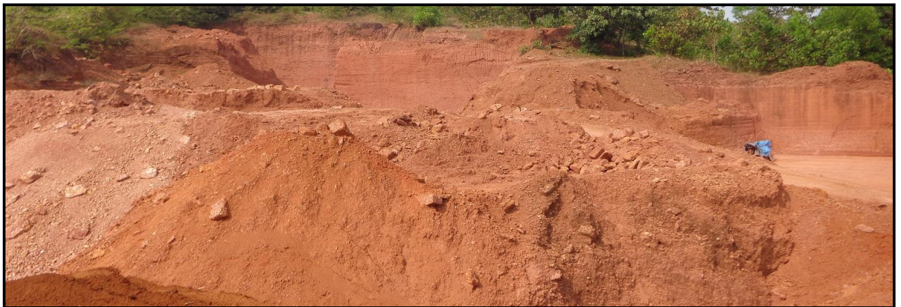
Photo 18: Slope modification through quarrying of lateritic soil for brick making near Dambe
